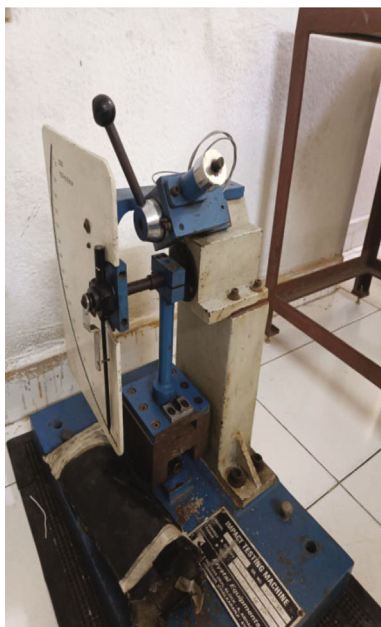
FIGURE 2: Setup of impact testing.
