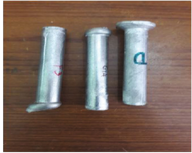
FIGURE 1: Casted LM25- \text{Fe}_3\text{O}_4 -Gr MMHCs specimen.
