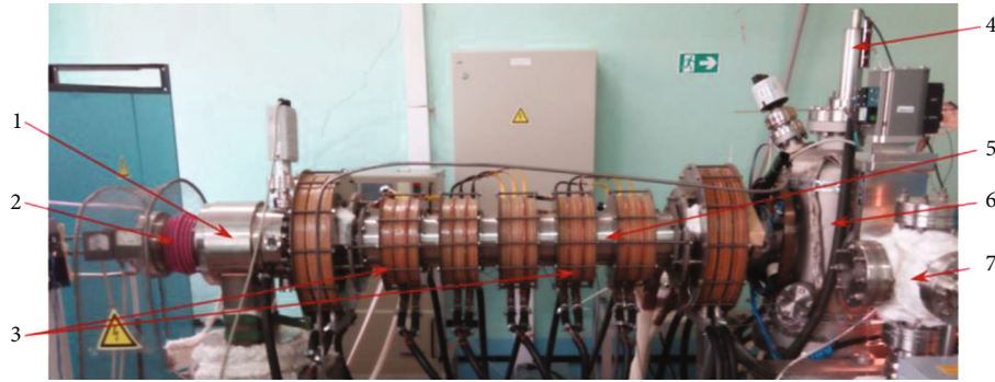
FIGURE 1: General view of the plasma-beam installation. (1) Electron beam cannon chamber; (2) electron beam cannon; (3) electromagnetic system; (4) Langmuir probe; (5) plasma-beam discharge chamber; (6) interaction chamber; (7) loading chamber.
