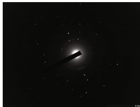
FIGURE 8: Selected area electron diffraction (SAED) pattern of gold nanostars obtained at pH 4.0 and collagen concentration of 0.05 mM (scale bar 5 nm).
