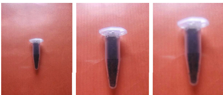
FIGURE 14: Silver nanoparticles of sizes from 25 nm to 35 nm, 55 nm to 65 nm, and 85 nm to 95 nm.
