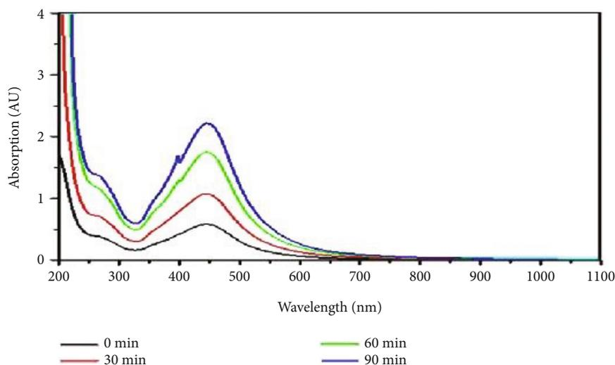
FIGURE 4: UV-vis spectral of AgNO<sub>3</sub> with *Fm*-ALE.
