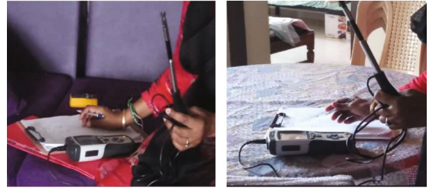
FIGURE 8: Reading taken with Hotwire Anemometer.
