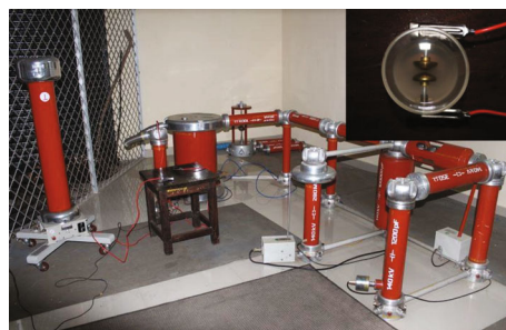
FIGURE 4: Photographs of the AC dielectric breakdown test setup and sample holder (inset picture).
