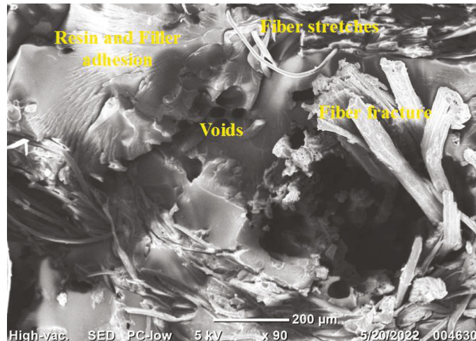
FIGURE 11: SEM image of the tensile-fractured surface bamboo fiber mat/coconut shell particle composite showing filler adhesion, voids, fiber fracture, and pull-out.
