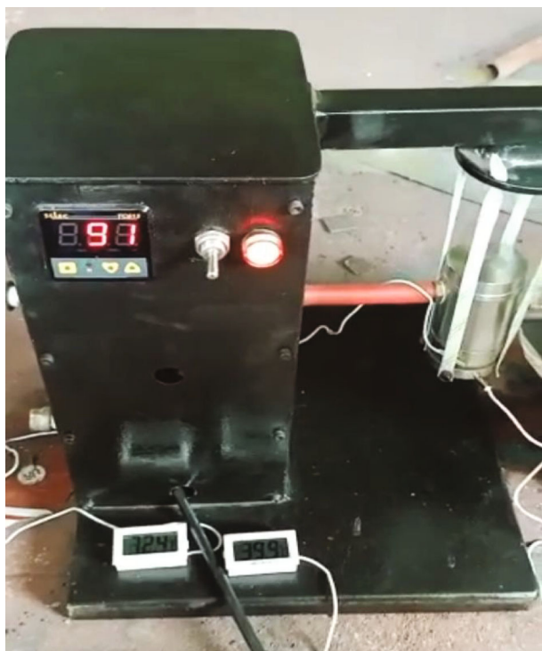
FIGURE 2: Thermal conductivity measurement by using Lee's disc method.
