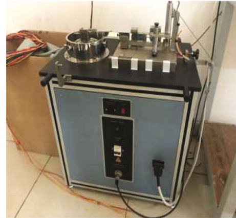
FIGURE 3: Pin on disc apparatus.
