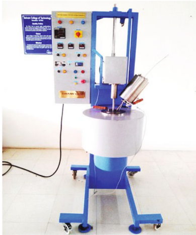
FIGURE 1: Experimental setup of stir casting furnace.
