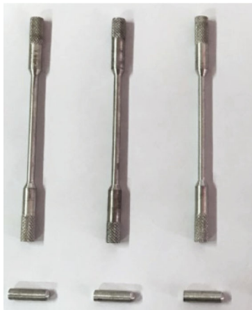
FIGURE 2: Fabricated tensile and wear samples.
