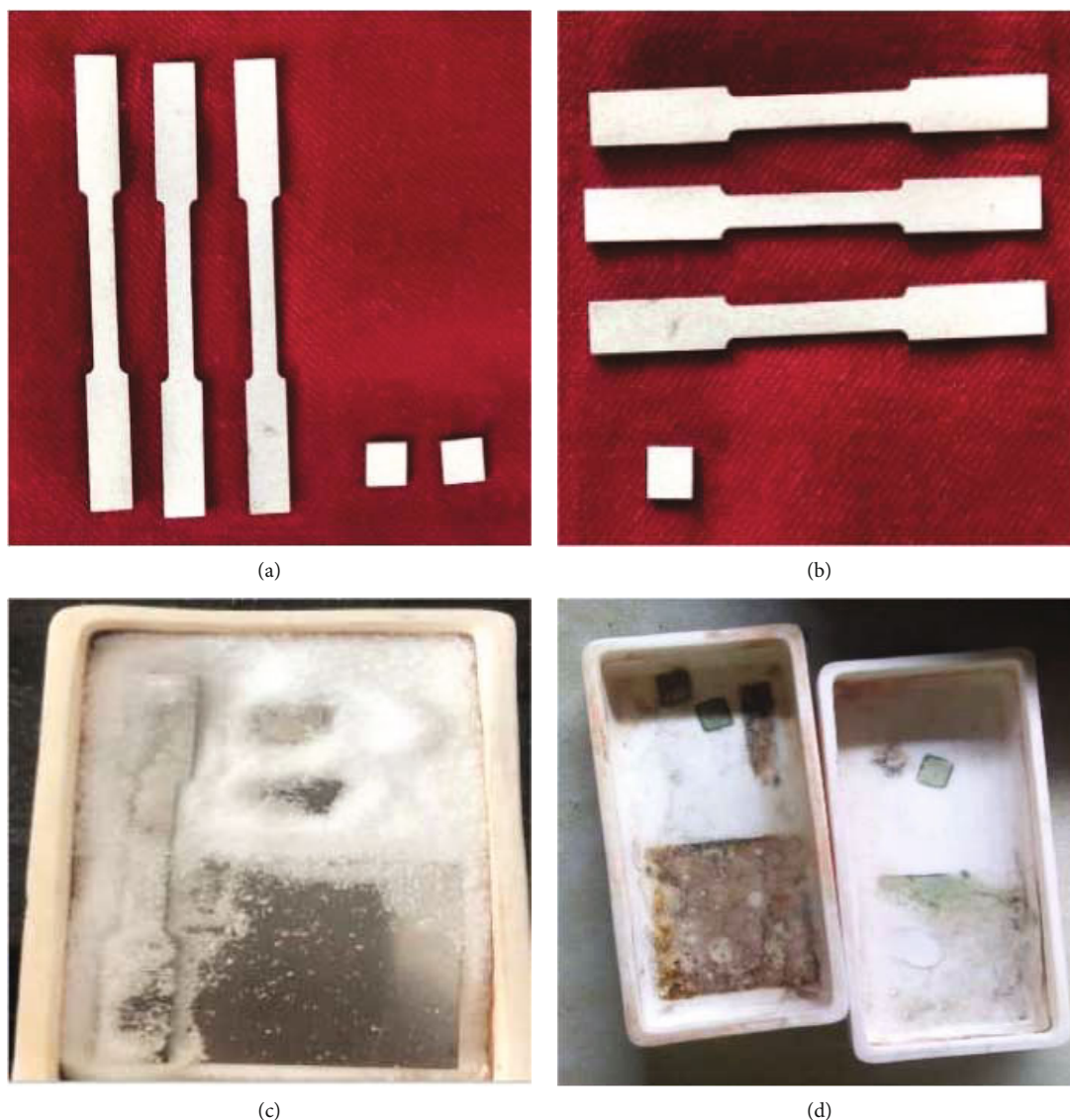
FIGURE 3: (a) YSZ-Inconel 625-coated specimens. (b) YSZ-Incoloy 800H-coated specimens. (c) Specimens before heating. (d) Specimens after heating.
