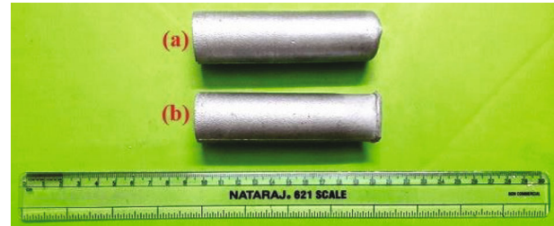
FIGURE 1: Squeeze casted specimen: (a) Ti-6Al-4V with 10 wt% WC composites; (b) Ti-6Al-4V with 15 wt% WC composites.
