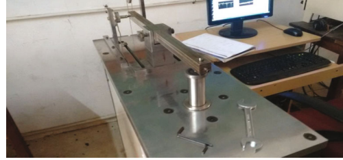
FIGURE 1: Pin-on-disc set-up used for dry sliding test.
