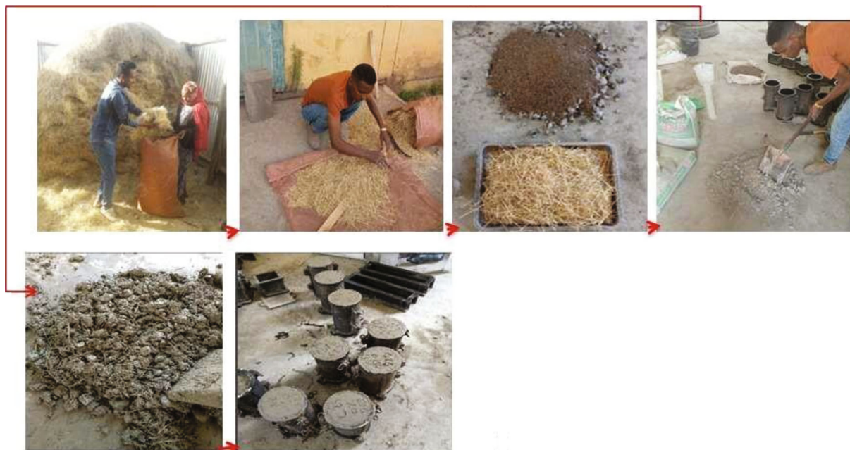
FIGURE 2: Teff-straw-collection techniques and specimen preparation process.
