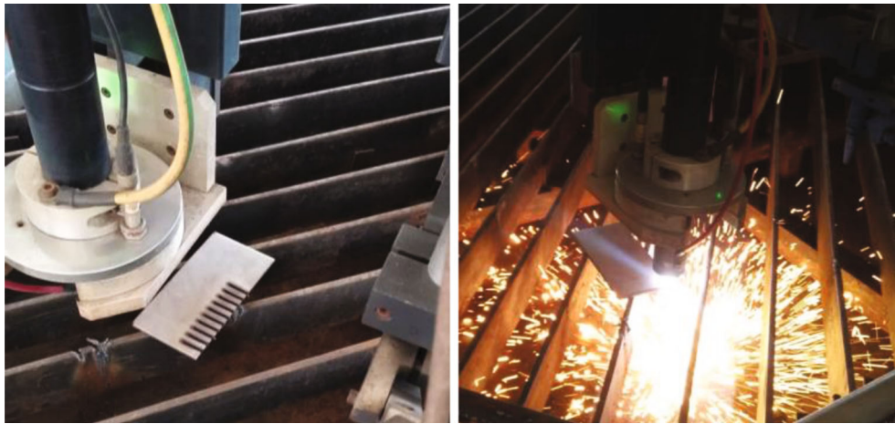
FIGURE 4: Plasma arc cutting of Inconel 718.
