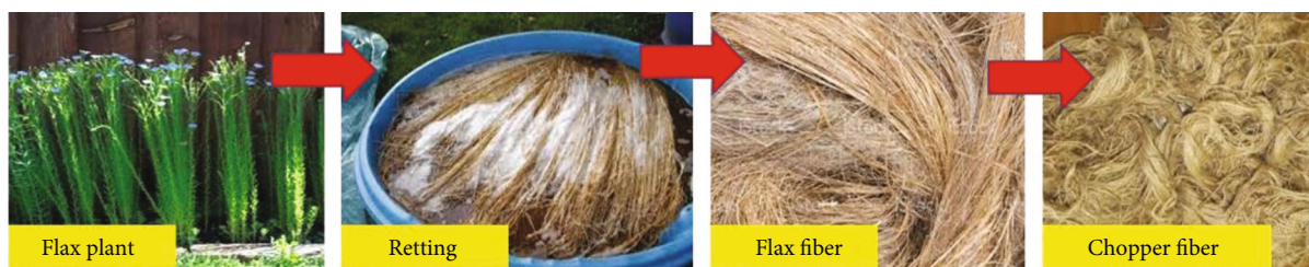
FIGURE 1: Flax fibre extraction from flax plant.
