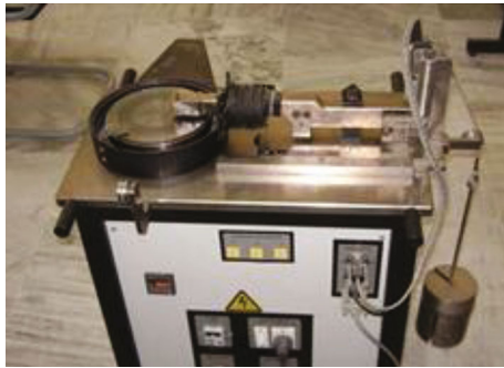
FIGURE 3: Wear testing arrangements in the pin-on-disc apparatus.
