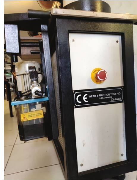
FIGURE 3: Pin-on-disc wear test apparatus.
