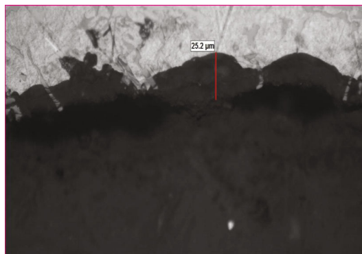
FIGURE 6: Microscopic photo of the oxide layer of the normal anodized sample.
