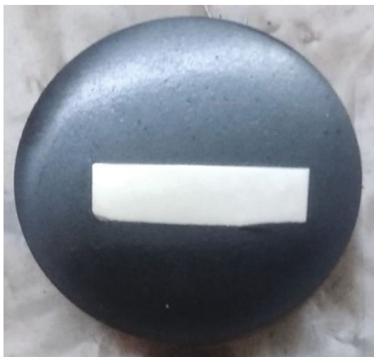
FIGURE 4: Mounted sample for measuring thickness of the oxide layer.
