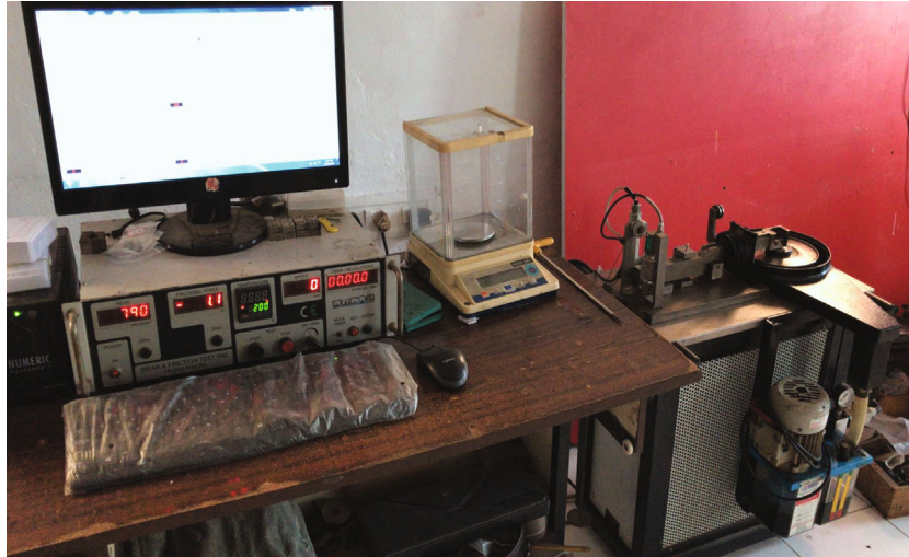
FIGURE 2: Pin-on-disc wear testing machine.
