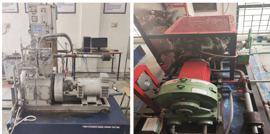
FIGURE 3: Experimental setup of diesel and petrol engine with fabricated SCR.
