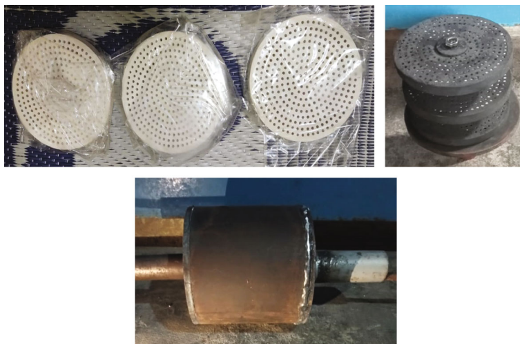
FIGURE 2: Fabrication of SCR catalytic converter.
