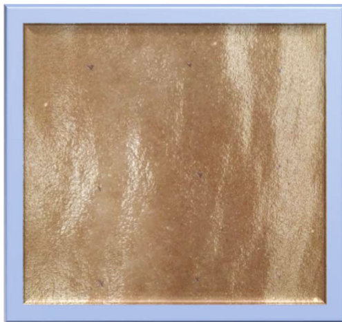
FIGURE 13: 1.25 wt.% CNF spray-coated wet laminates of cellulose nanofiber on the paper.
