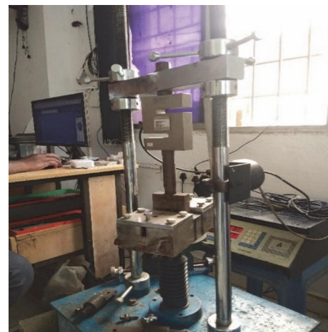
FIGURE 6: Interlaminar shear test setup.
