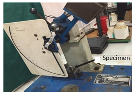
FIGURE 7: Izod impact test setup.
