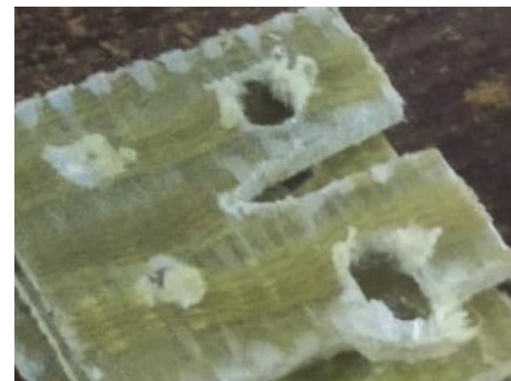
FIGURE 19: A test specimen undergone Mode-1 fracture test.
