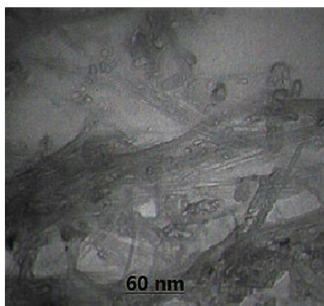
FIGURE 4: TEM images of PEG-PEI-SWCNTs with a rough tubular structure. Some particles appeared to be attached and distributed along the SWCNT sidewalls, indicating that PEG and PEI are conjugated onto nanotube. Scale bar: 60 nm.
