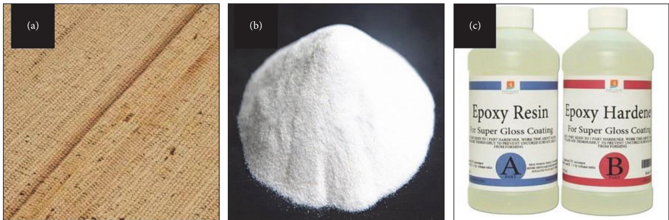
FIGURE 1: Photographic image of (a) banana fiber; (b) nano-SiO 2 ; (c) epoxy matrix materials.
