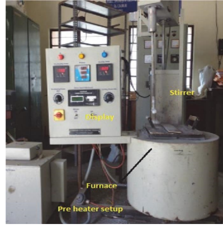
FIGURE 1: Stir casting arrangement.
