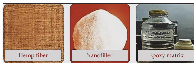
FIGURE 1: Photographic images of reinforcement, filler, and matrix materials.
