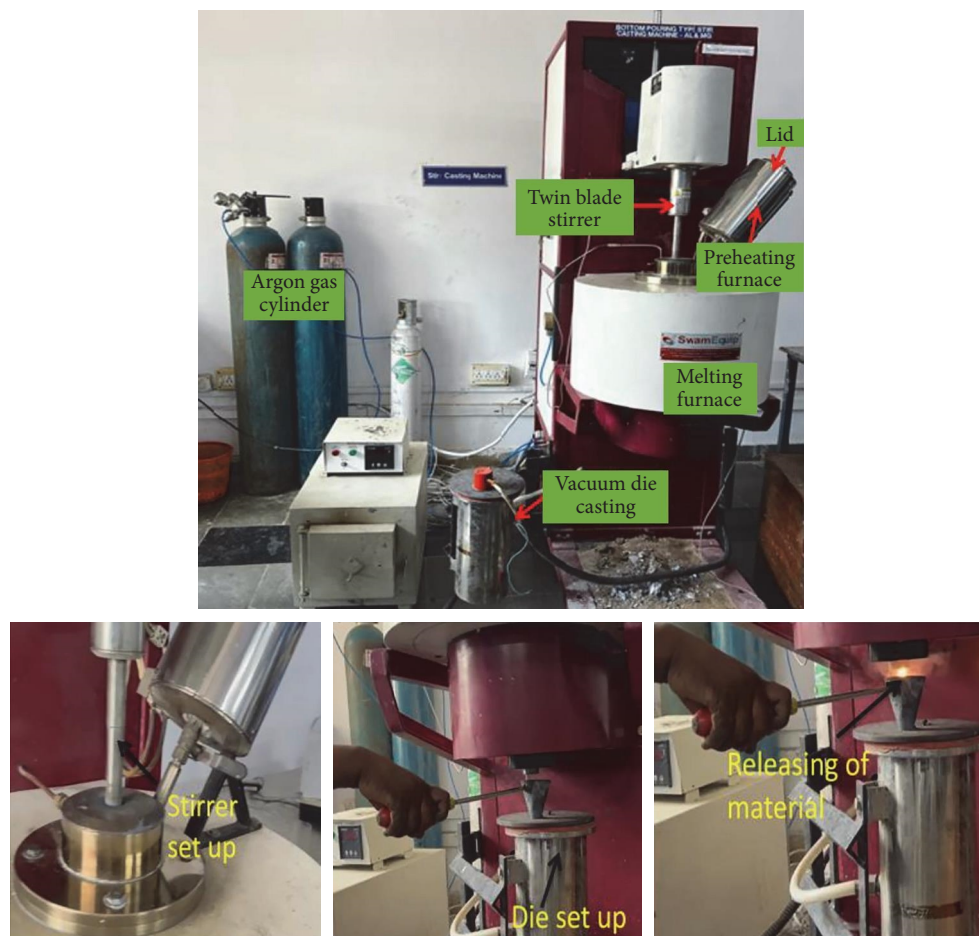
FIGURE 1: Stir-casting set up.
