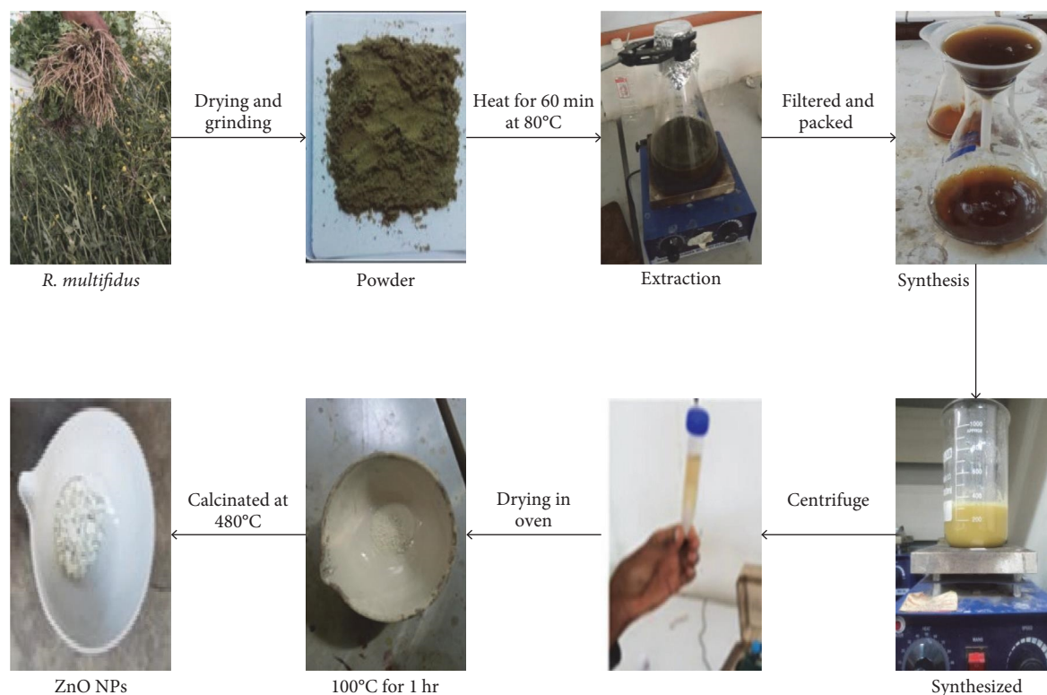
FIGURE 1: A schematic of the synthesis of ZnO NPs using Ranunculus multifidus plant extract.
