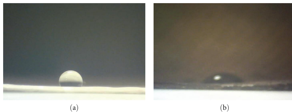
FIGURE 6: Contact angle measurement for pristine (a) and modified (b) 1 hr PA PVDF membrane.
