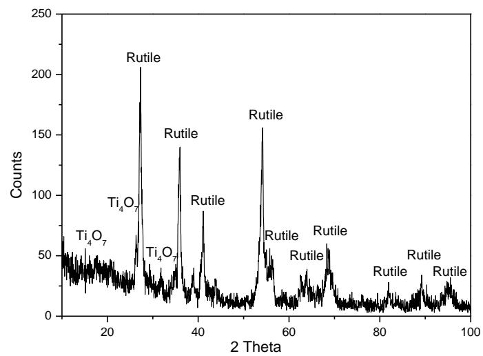
**Figure S1.** XRD patterns of Nb-TiO<sub>2</sub> sphere support.
