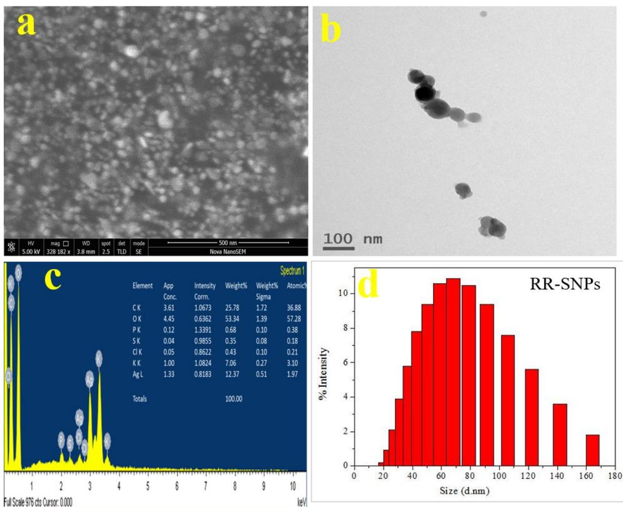
**Figure S1.** Spectroanalytical characterization of biogenic RR-SNPs: (a) SEM micrograph (b) TEM image (c) EDX Spectrum (d) Histogram of particle size distribution.
