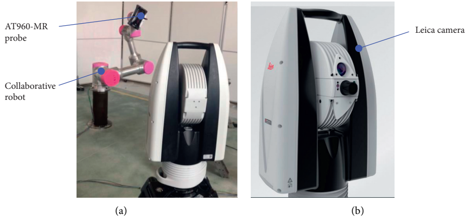
FIGURE 3: Experimental layout and front view of Leica measuring equipment.
