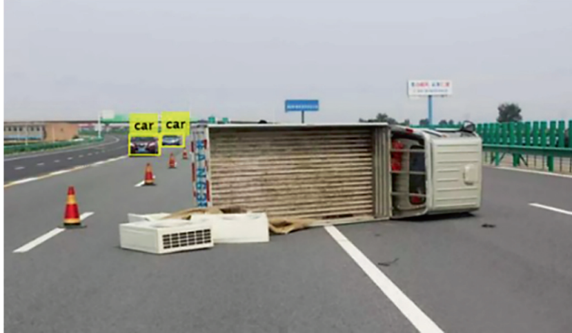
FIGURE 1: Fast R-CNN. Normal cars are detected, but the overturned car and the box are not detected.
