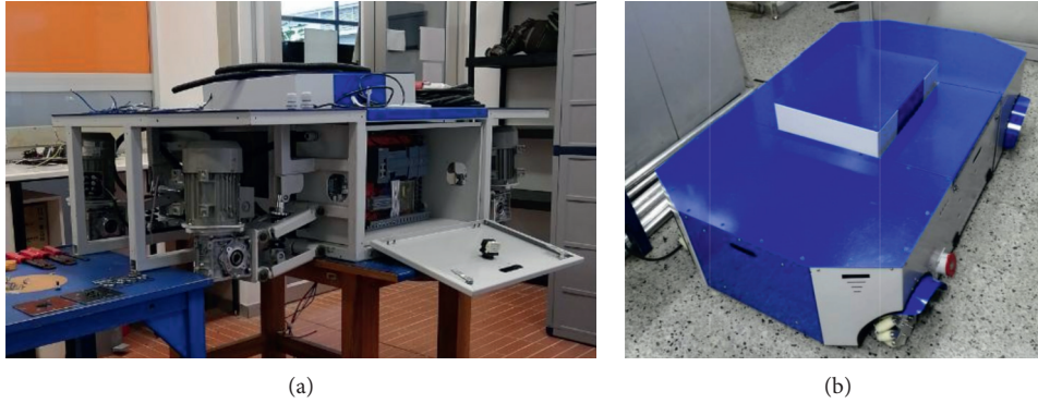
FIGURE 14: (a) Real AGV prototype during assembly and (b) final prototype.
