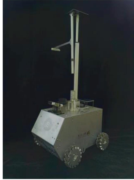
FIGURE 1: Overall structure of the robot. (1) Multi-terrain replacement chassis. (2) Surveillance camera. (3) Lidar. (4) Camera module. (5) Electronic control lift image acquisition bracket. (6) Car display. (7) Quick release mechanism.
