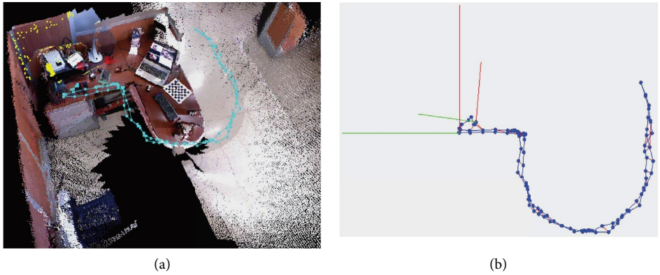
FIGURE 12: Map made with RTAB-Map. In (a), the dense point cloud gives the model a realistic appearance. The position graph in (b) shows the edges or estimated trajectory of the camera (line segments in blue), nodes (blue points), and the detection of closed loops (line segments in red).
