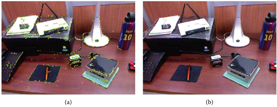
FIGURE 13: Visual odometry (a) and closed loop detection (b) carried out by the RTAB-Map system.
