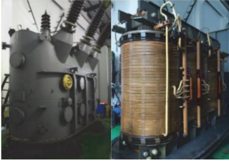
FIGURE 1: The structure of the oil-immersed transformer.
