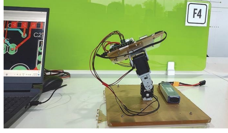
FIGURE 9: Experimental setup to analyze and validate the attitude estimator.
