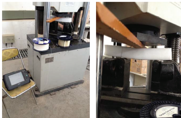
FIGURE 13: Bending experiment of the composite monitoring device.
