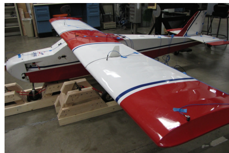
FIGURE 1: The Super Hauler in the test rig while instrumented with accelerometers.
