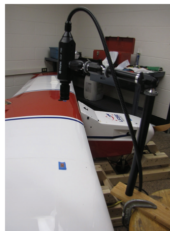
FIGURE 2: Test setup with the laser vibrometer measuring the response of the UAS.
