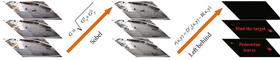
FIGURE 3: Left-behind baggage detection. When the separation of human and objects is detected, the item would be marked out. When a pedestrian leaves the monitored area, the model outputs it as an abnormal behavior.
