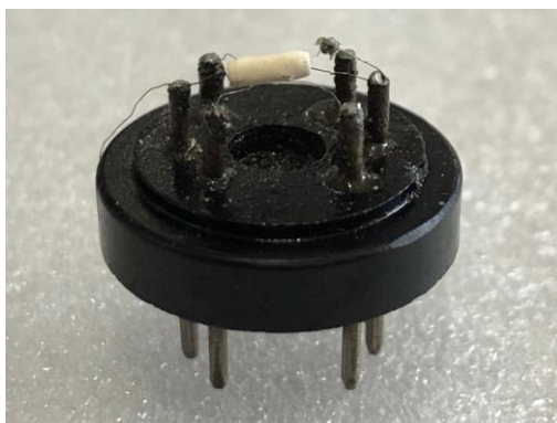
Figure S1: gas sensor used for characterizing gas sensing behavior of samples
