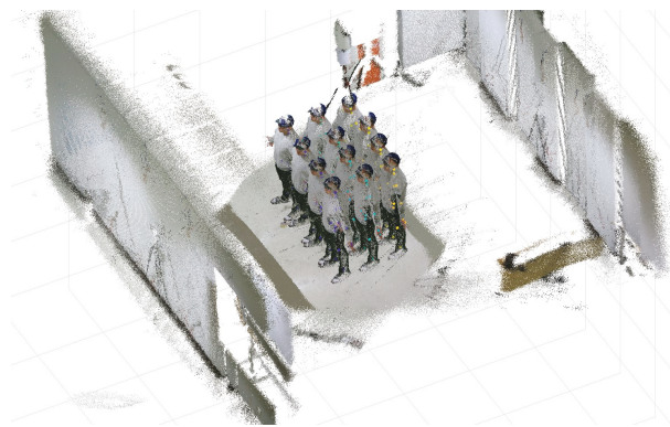
FIGURE 13: 12 positions of the standing person as a calibration target for acquiring multiple skeleton data.
