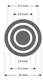
FIGURE 1: Tripolar concentric ring electrode with dimensions of its central disc, middle ring, and outer ring.
