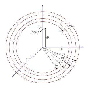
FIGURE 2: Four-layer concentric inhomogeneous spherical head model with the radii of the layers equal to R = 8.8 cm, dR = 8.5 cm, cR = 8.1 cm, and bR = 7.9 cm and the conductivities of the layers equal to  $\sigma_1 = 3.3 \times 10^{-3}$ ,  $\sigma_2 = 10.0 \times 10^{-3}$ ,  $\sigma_3 = 4.2 \times 10^{-5}$ , and  $\sigma_4 = 3.3 \times 10^{-3}$  S/cm, from inside to outside, respectively.
