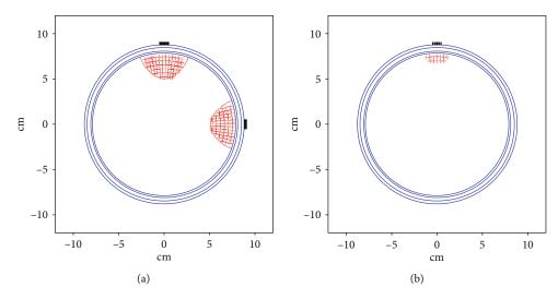
FIGURE 3: The red (hashed) lines show the HSV of conventional disc electrodes (a) and TCREs (b).
