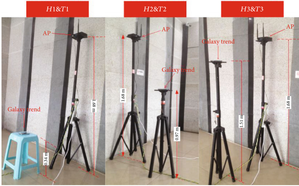
FIGURE 5: Configuration of the heights picture. H1 vs. T1 , H2 vs. T2 , and H3 vs. T3 .
