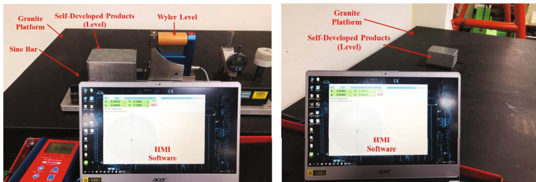
FIGURE 9: Experimental setup for repeatability and stability measurement.
