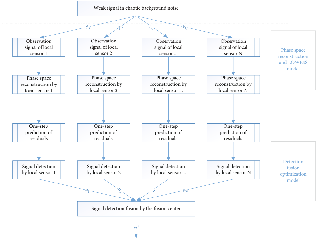
FIGURE 2: Schematic diagram of detection fusion of weak signal under chaotic noise.
