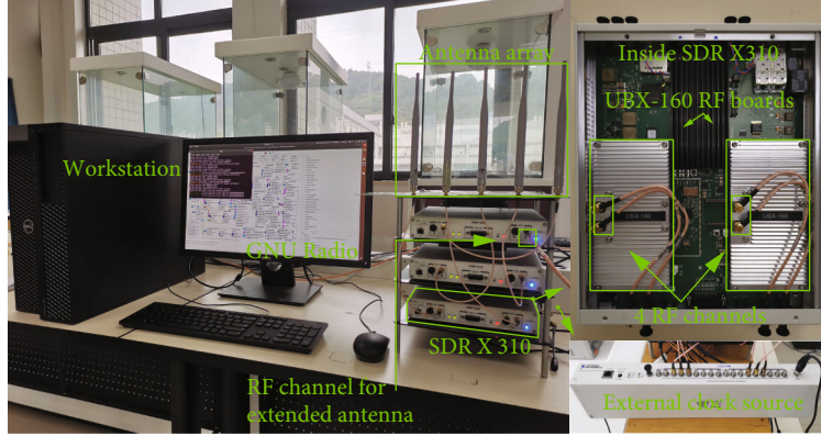
FIGURE 2: The receiver of the SDR test platform. The receiver is composed of three independent X310, which can provide 6 RF channels to receive the wireless signal, and the signal bandwidth can reach up to 100 MHz.
