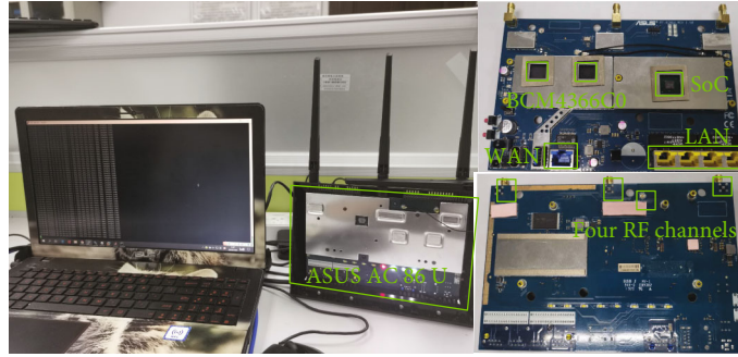
FIGURE 4: The receiver of the IEEE 802.11n protocol-based Broadcom 4366C0 test platform. This receiver can provide 4 RF channels to receive the wireless signal and the signal bandwidth can reach up to 80 MHz.
