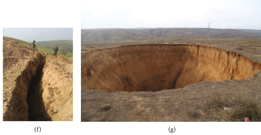
FIGURE 1: (a) Study area position on the map of China with the location of Ordos marked with a red line. (b) The location map of the coal mining area; the green and yellow lines represent SAR image coverage; the red line represents coal mining area. (c) The latest Google Earth image of the study area. (d) Coal mine area (SRTM 30 m resolution) elevation map. (e–g) Surface cracks and collapse pits in the study area.
